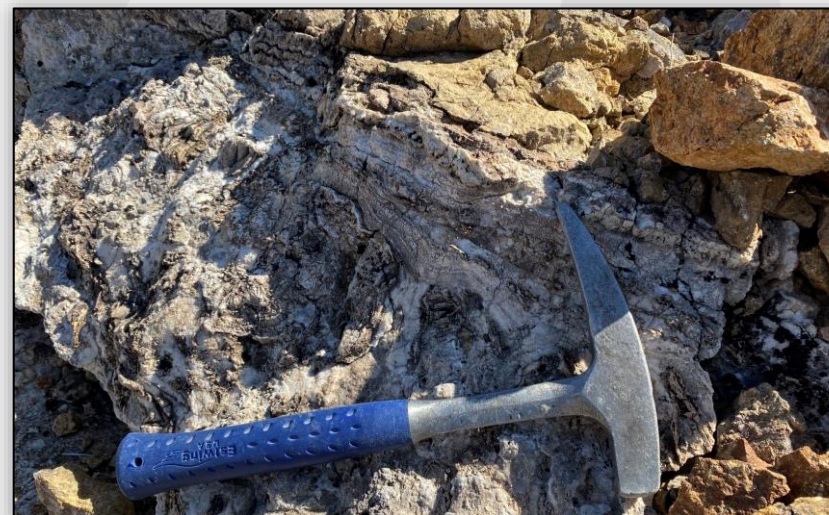
Multi-phase quartz-calcite-chalcedony-adularia vein breccia cut by banded quartz-calcite-adularia vein – Apex prospect, Mohave Project
