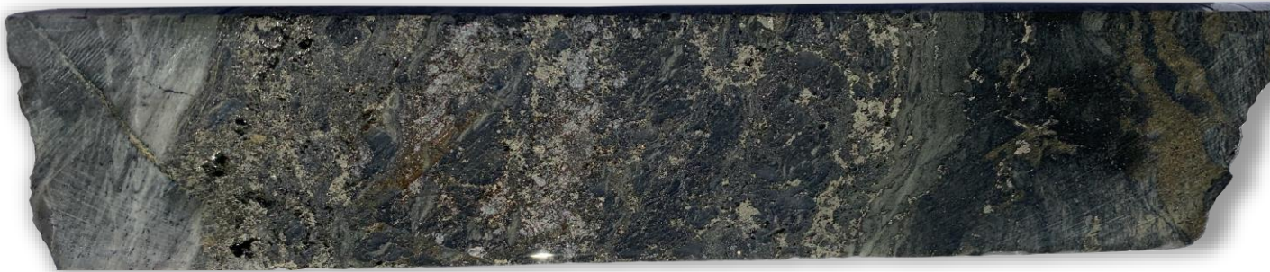
DD21GC034 – Sulphide replacement style mineralization – pyrite-arsenopyrite.
