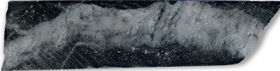
DD21GC035 – “Needle” arsenopyrite with fine visible gold.
