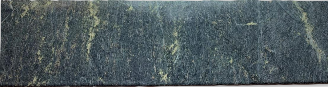
DD22SK002 – Abundant pyrite-chalcopyrite in sheared mafic volcanics.
