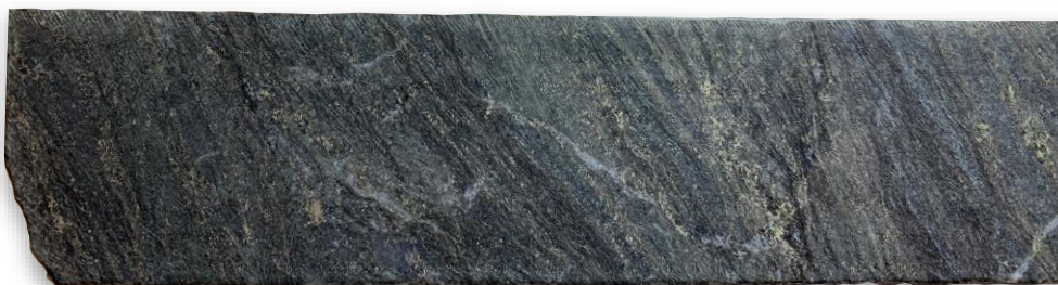
Silica-biotite-chlorite altered mafic volcanic with abundant fine disseminated pyrite – Skinner drill core
