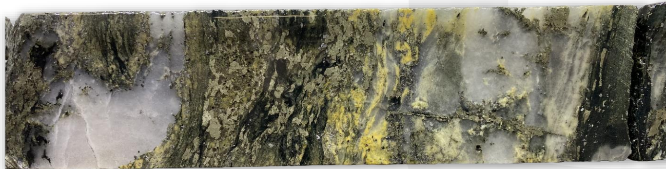
Drill core from 2021 Golden Corridor drilling – Pyrite with fine visible gold in quartz carbonate vein – Golden Sidewalk Project
