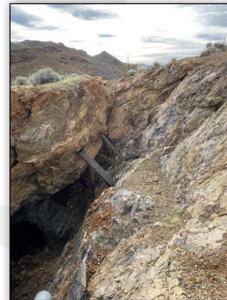
Dixie Mine prospect: Stope developed on sheeted calcite-quartz veinlets – 0.5 m @ 9.22 gpt Au
